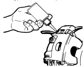
Any excess grease that squeezes out from the mating surfaces should be removed.
